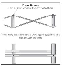
Herringbone strutting should only be used where the spacing of the joist does not exceed three times the joist depth. Manufactured from galvinised mild steel to BS EN 10142: 1991, DX 51D+Z275.
